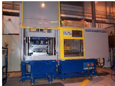
Figure 1 The Dasset compression extrusion rig
