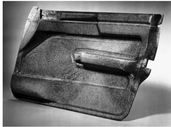
Figure 10: Car door interior panelling from biocomposites, manufactured at the DLR
